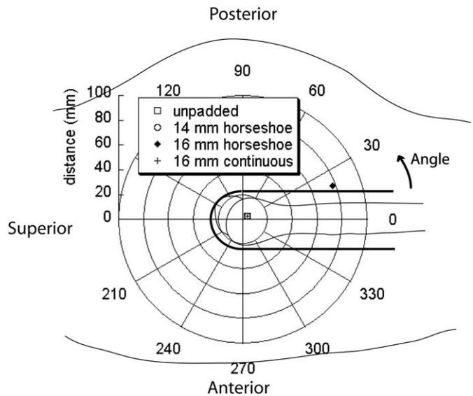
**Fig. 4.** Changes in the location of peak pressure as function of hip protector types (all for 20 cm drop height and placed in their intended location). Peak pressure was shunted away from the danger zone by the 16 mm horseshoe protector, but with both 14 mm horseshoe and 16 mm continuous protectors the peak pressure remained within the danger zone and its location did not change. Note that the unpadding, 14 mm horseshoe and 16 mm continuous data points all overlap and are centered on the GT.
