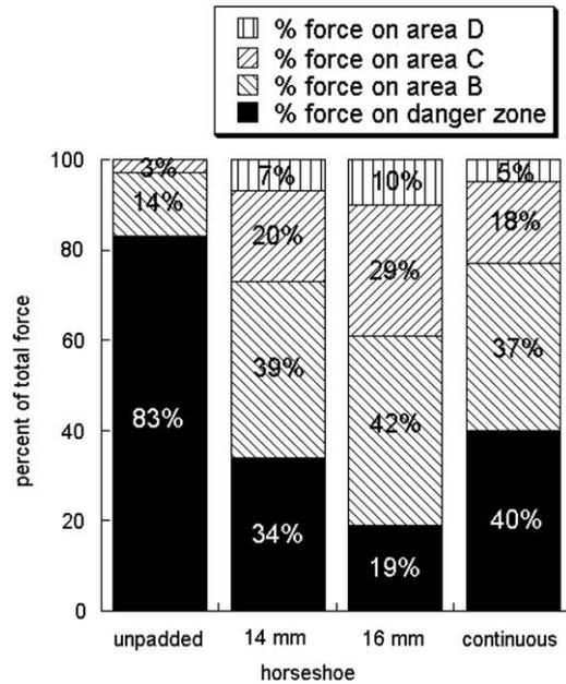
**Fig. 5.** Force distribution to four different areas over the hip. For a 20 cm drop height, the force applied to the danger zone was 83% of the total force in the unpadding condition, but only 19% of the total force with the centrally placed 16 mm horseshoe protector.
